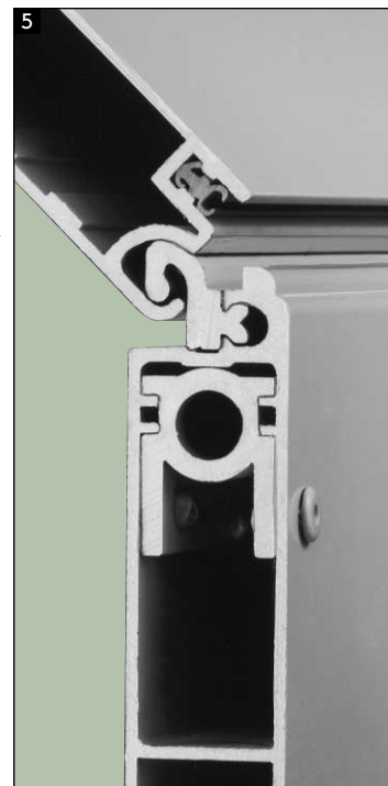
Joint seal between panels. Channel extruded into bottom of upper panel meshes with tongue-and-groove feature prevents damage to joint by absorbing any impact loads that may occur.
