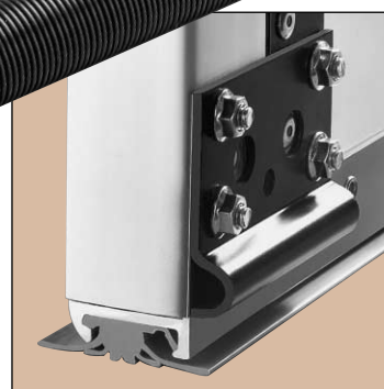
3 All panels are equipped with PVC end caps. Removable bottom roller bracket designed for easy roller replacement.
