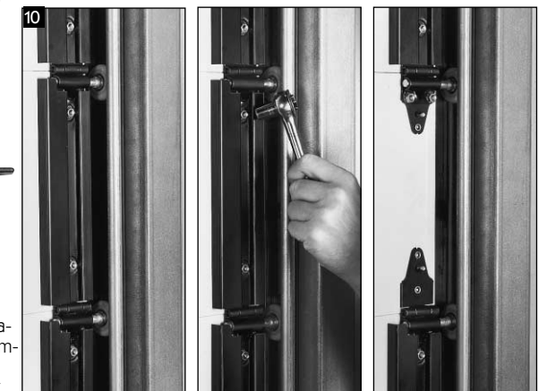
10 Patented CargoGuards form vertical rubrails to shield hardware from shifting freight. Covers are easily removed to access hinges and rollers.
