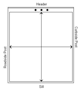
Measure the opening WIDTH of your truck or trailer (distance between roadside post and curbside) and the opening HEIGHT (distance between header and sill as shown).
